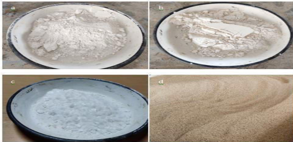
Figure 1: (a) calcined clay (b) GGBS (c) flakes of sodium hydroxide (d) fine aggregate
