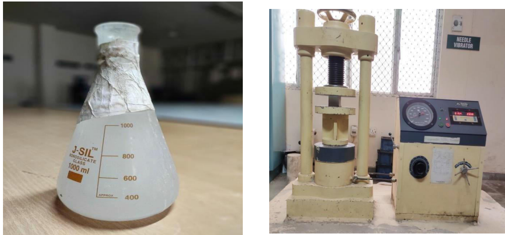
Figure 2: (a) Solution of sodium hydroxide (b) compression testing machine
